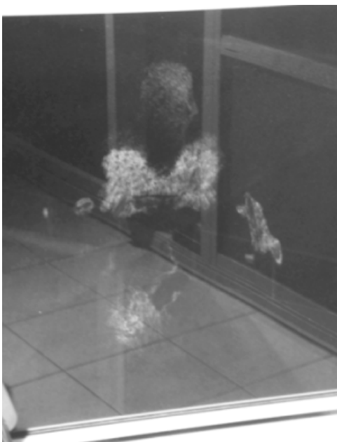
FIG. 1—Imprint on outside of the glass panel viewed from inside the apartment. The photograph shows the entire 1.0 m high glass panel from the balcony rail at the top of the photo to the balcony floor at the bottom of the photo.
